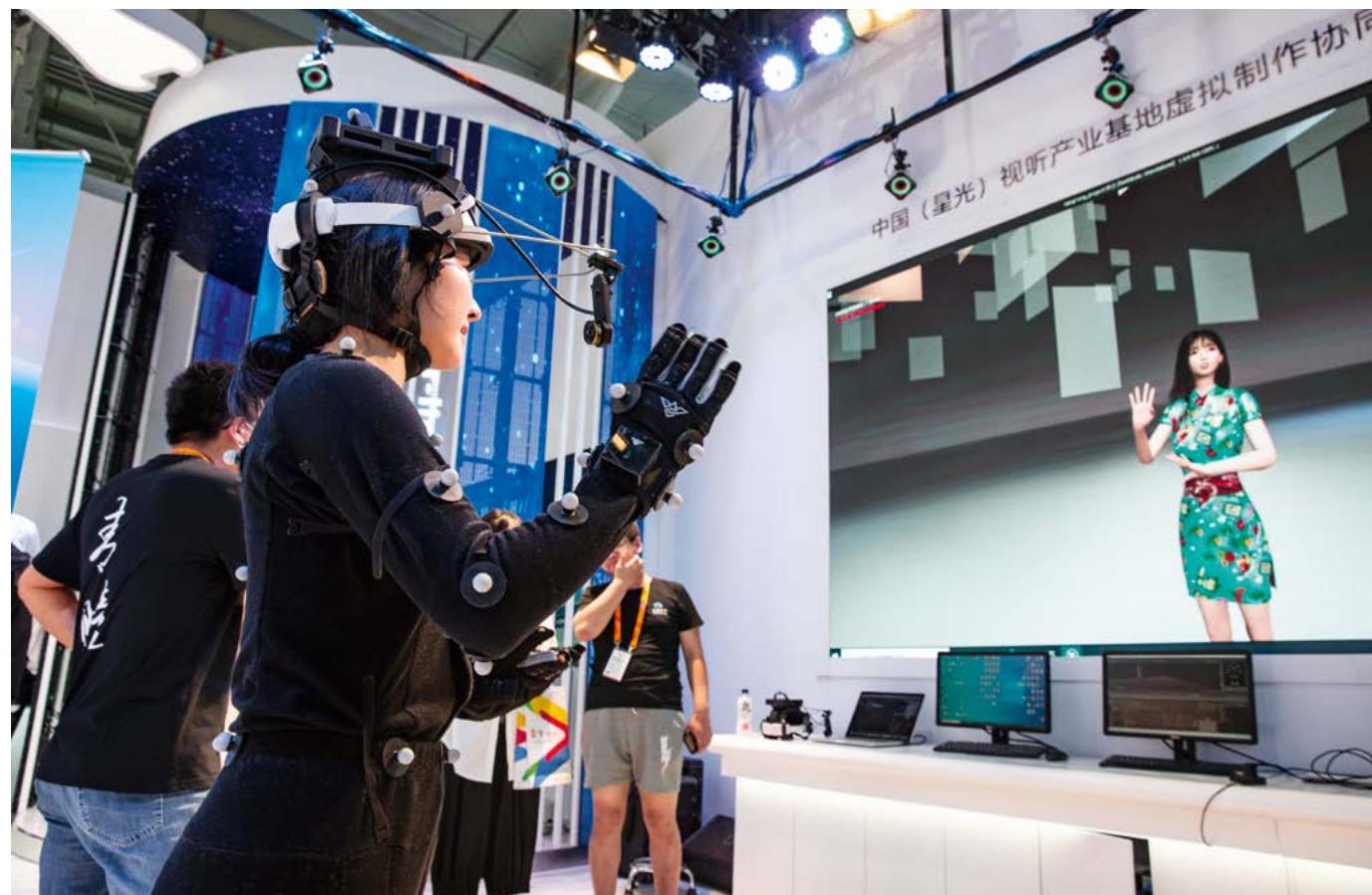
The metaverse experience area of the China International Fair for Trade in Services held in Beijing showcases an optical motion capture system, September 2, 2022. This technology enabled the virtual dancer on a large screen to mirror the body movements of the experimenter. (Photo by Qin Bin/China Pictorial)
